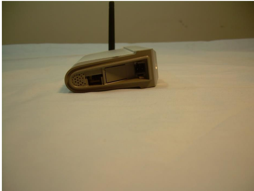
Photograph 10 – View of the Side of the EUT Showing Power Port
