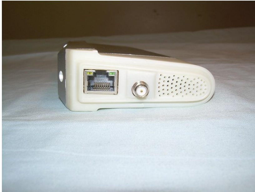
Photograph 9 – View of the Side of the EUT Showing Antenna Connector and Ethernet Port
