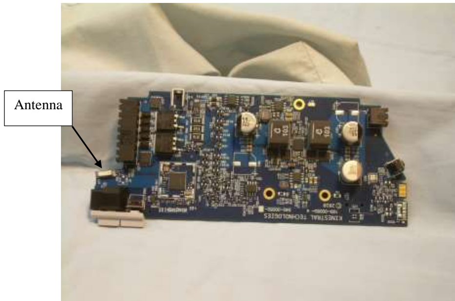
Photograph 11: Top Side of the PCB with Heatsink Removed
