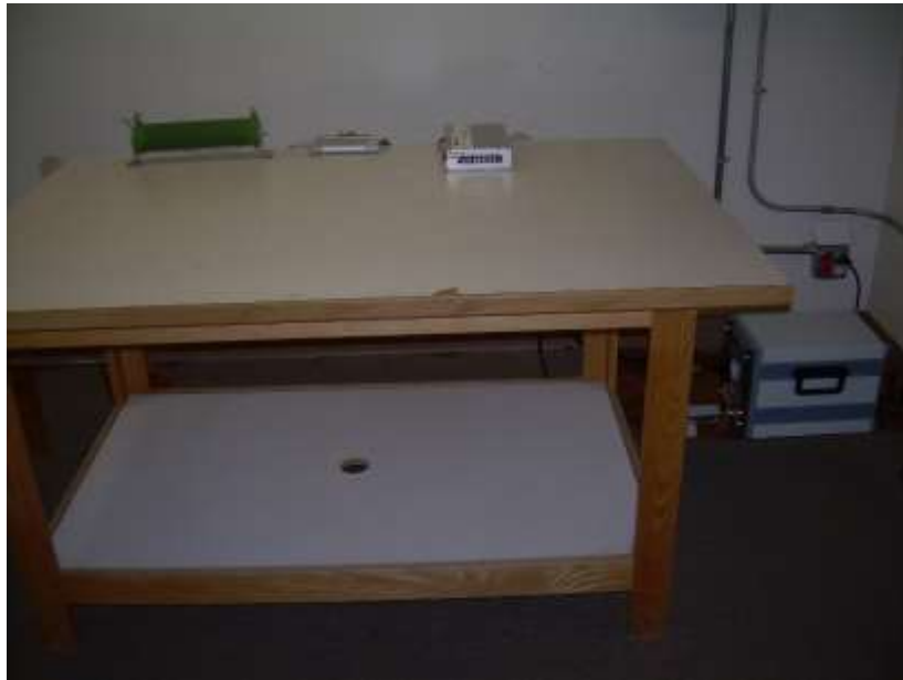
Photograph 4: Front View Conducted Emissions Worst Case Configuration
