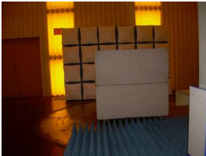
Photograph 2: Front View Radiated Emissions Worst-Case Configuration – Below 1000 MHz
