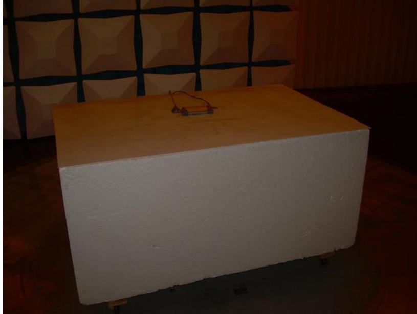
Photograph 1: Front View Radiated Emissions – Below 1000 MHz Configuration
