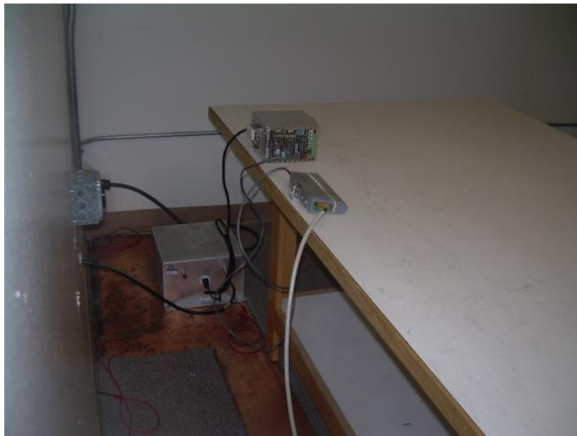
Photograph 6: Back View Conducted Emissions Worst-Case Configuration
