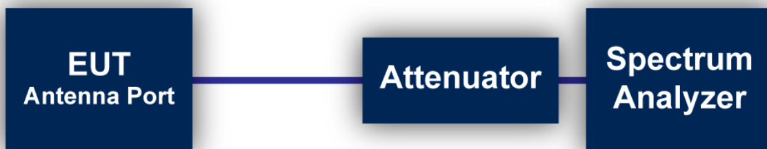
Figure 2: Direct Connection at the Antenna Port Test
