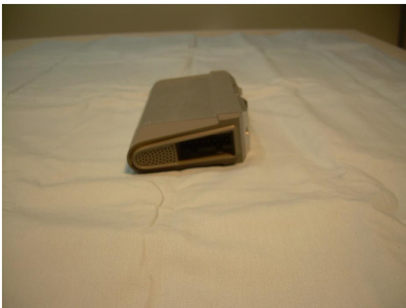
Photograph 10 – View of the Side of the DR200 Showing the Window Drive Interface Port
