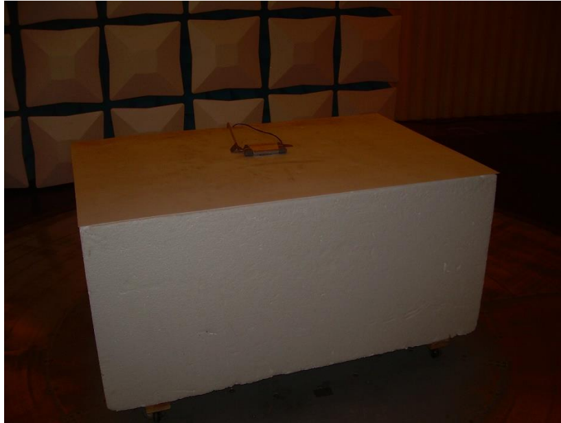
Photograph 1: Front View Radiated Emissions Configuration – Below 1000 MHz
