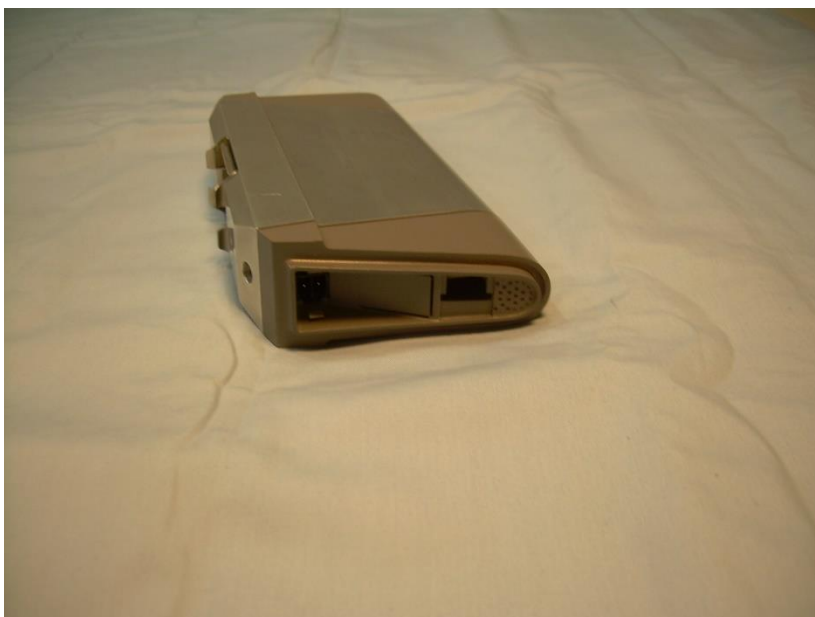
Photograph 9 - View of the Side of the DR200 Showing the Power Port
