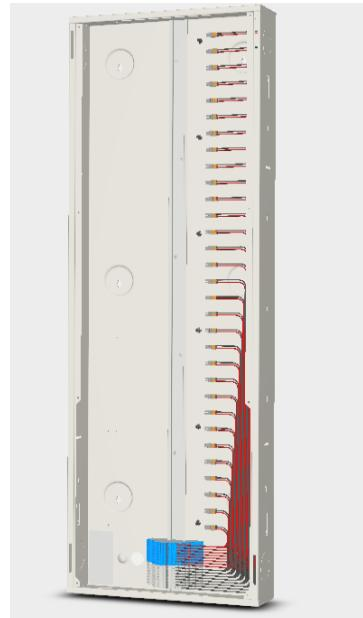
1. Use #8 screws rated for at least 100 lbs (45kg) loads. If installing on drywall, ensure the fasteners are driven securely into studs. If needed, a  $\frac{3}{4}$ -inch plywood back board can also be used to provide a rigid mounting surface spanning across studs.
