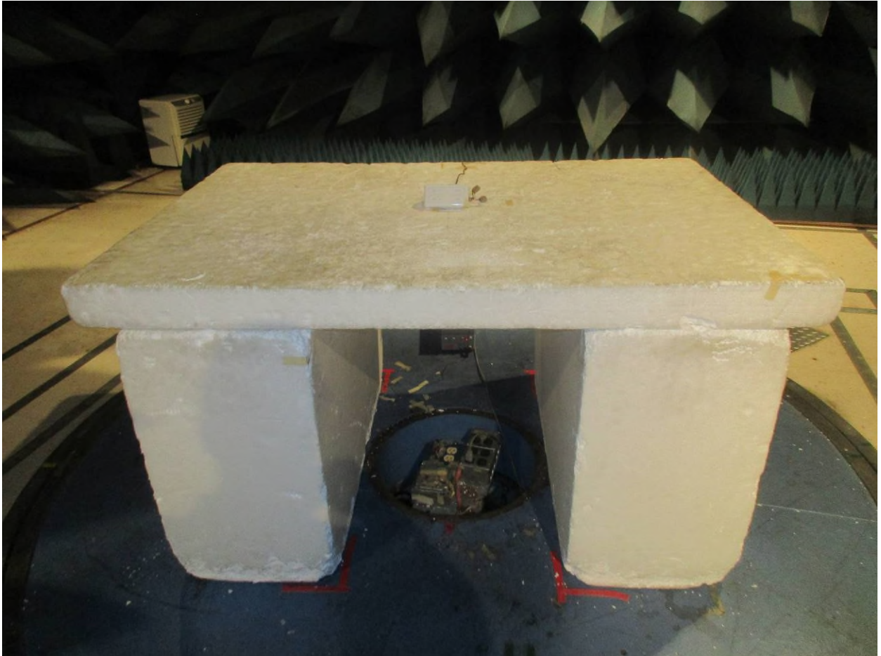
Figure 19: Radiated Emissions – Front View – below 1 GHz – EUT with Alternate Back Cover
