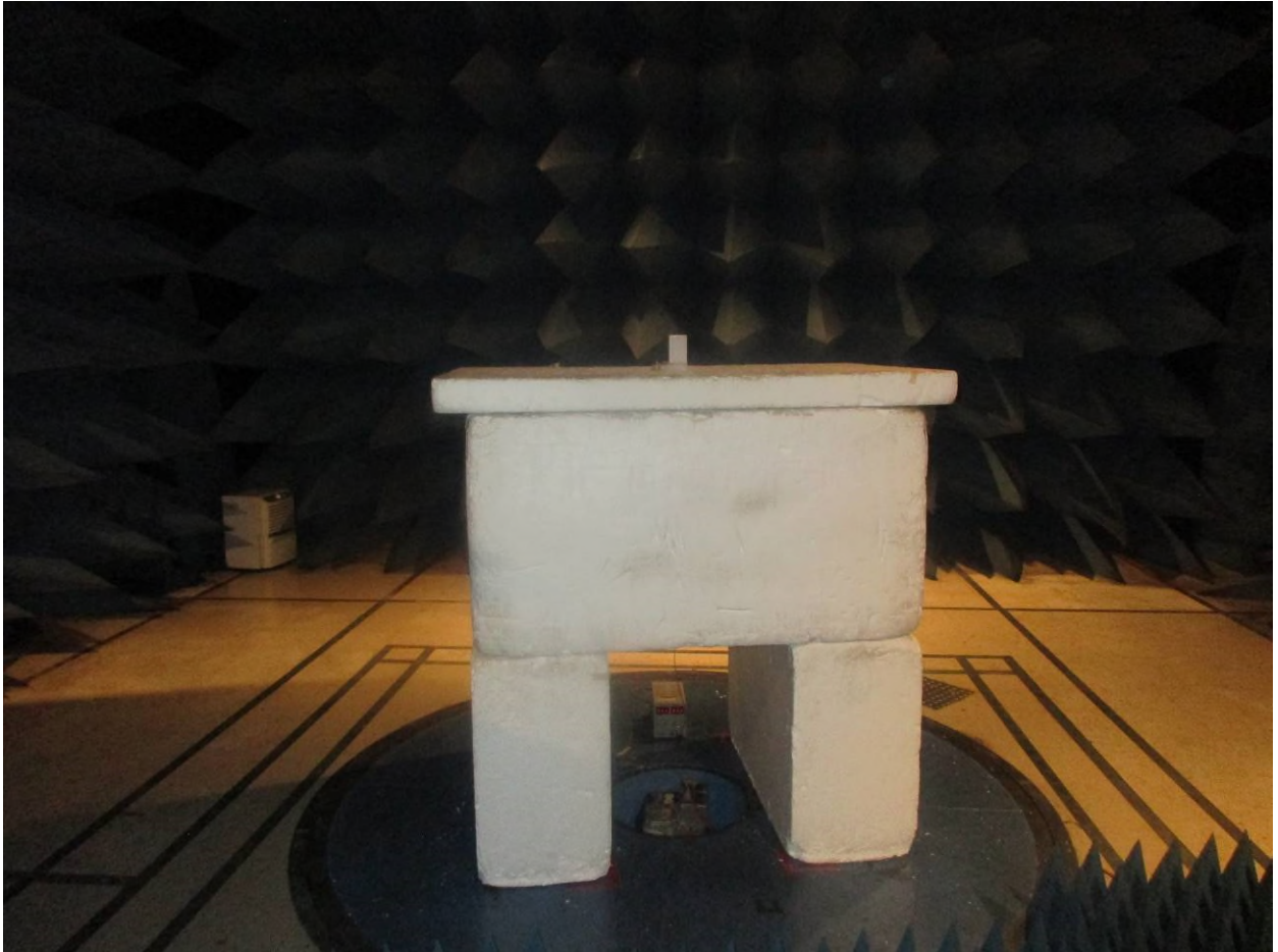
Figure 5: Radiated Emissions – Front View – above 1 GHz – EUT on Side
