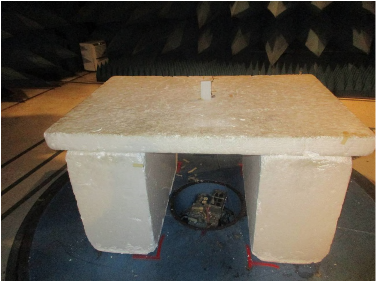
Figure 1: Radiated Emissions – Front View – below 1 GHz - EUT on Side
