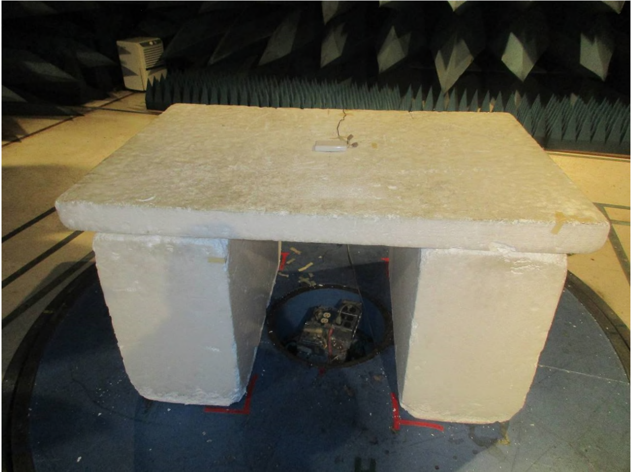
Figure 7: Radiated Emissions – Front View – below 1 GHz – EUT Flat
