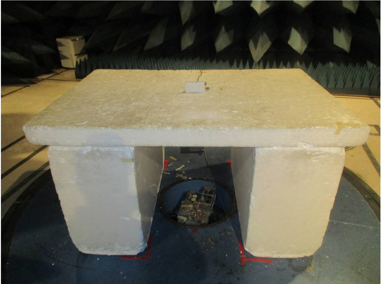
Figure 13: Radiated Emissions – Front View – below 1 GHz – EUT Vertical
