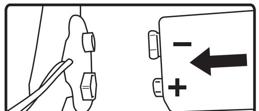
Using a Phillips head screwdriver, remove the bottom battery cover of the Base Station and Walkie Talkies. Insert 1 "9V" size battery (not included) in each in the polarity direction shown in the diagram. Replace the battery cover and tighten the screw.
