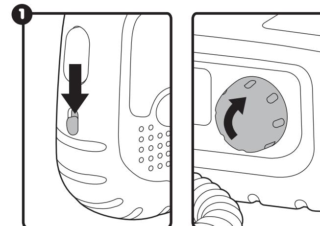
Slide the Walkie Talkie Switch down to turn the Walkies ON. Rotate the Base Station Knob clockwise to turn Base Station ON. The knob is also used to control the volume of the Base Station.
