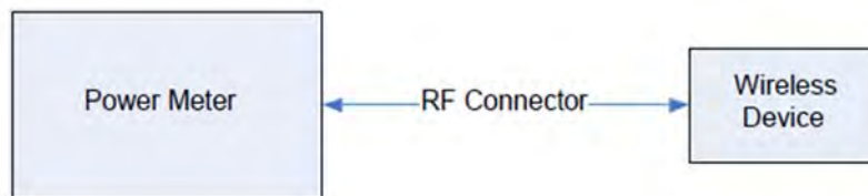
Figure 6.1.1 Power Measurement Setup
