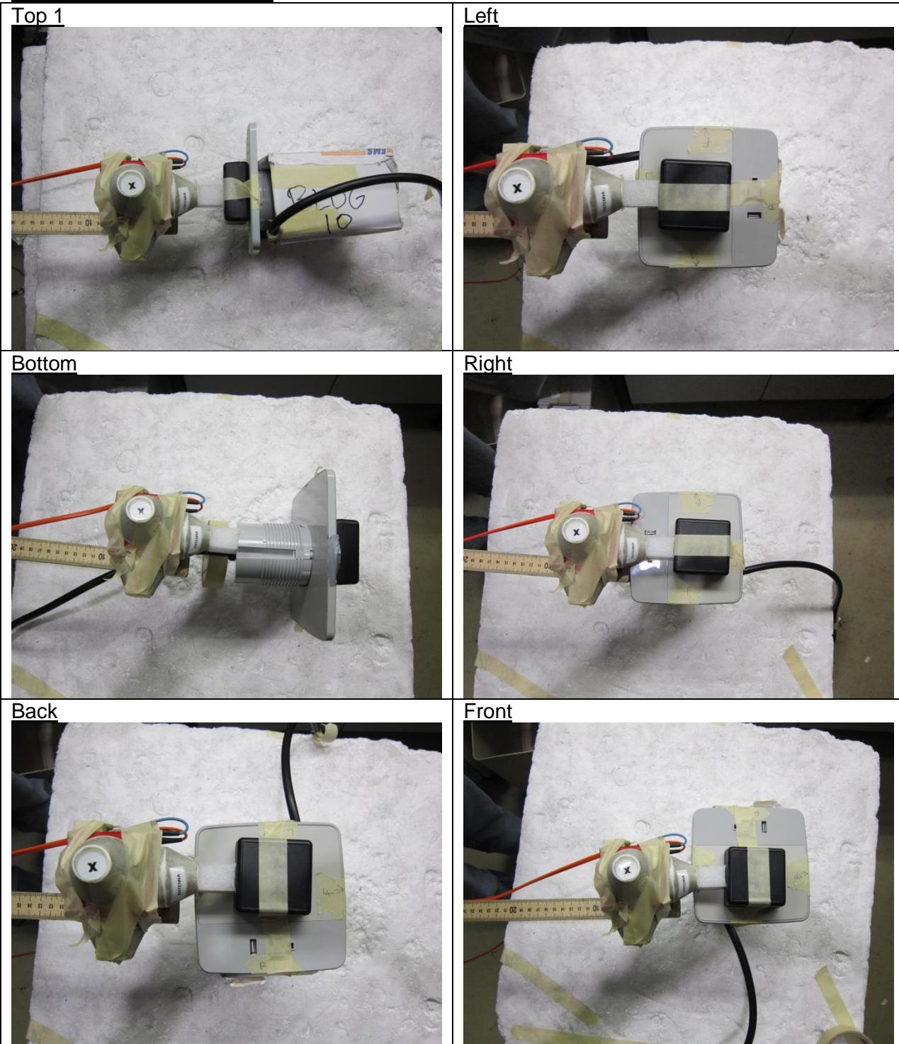
\* Foam spacer was added to probe edge. The distance between the reference of the probe and edge of the spacer is equal to 10cm. In photos above the ruler was used as non-conductive means to support the probe.
