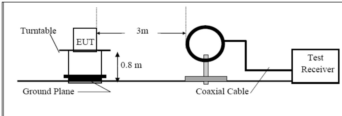
For Radiated Emission 30~1000MHz
