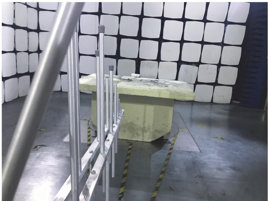
Radiation Emission Test Setup (30MHz to 1GHz)
