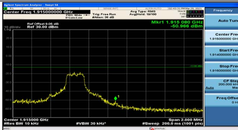
(Channel Bandwidth: 5 MHz)_HCH_QPSK_1RB#12
