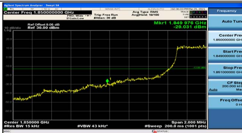
(Channel Bandwidth: 1.4 MHz)_LCH_QPSK_6RB#0
