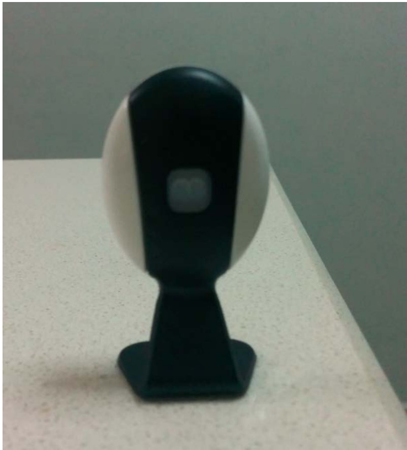
AllBe1 PIR sensor special bracket for human detection
