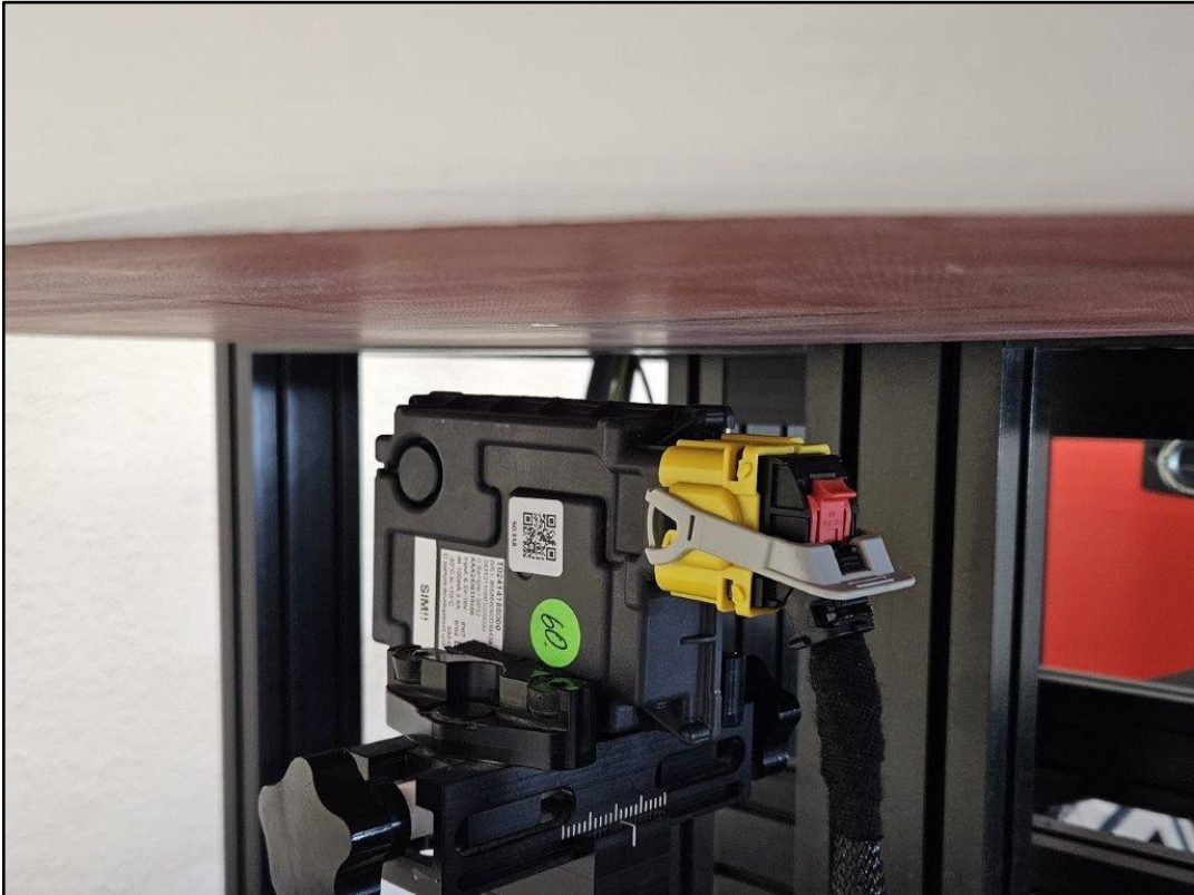
Photo 5: Test position left side with 20 mm distance
