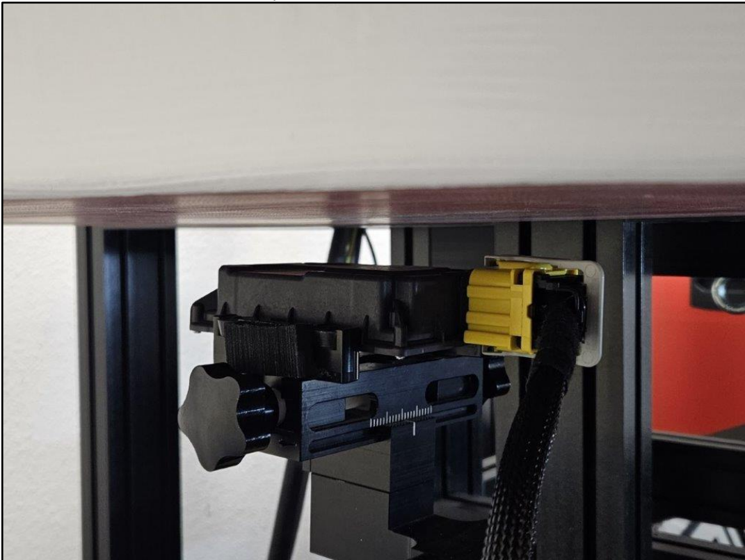
Photo 4: Test position front side with 20 mm distance
