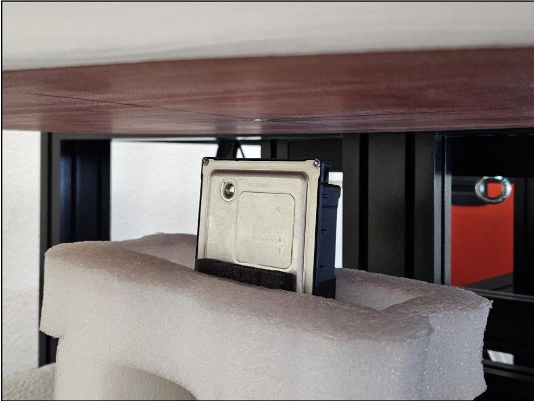
Photo 7: Test position bottom side with 20 mm distance
