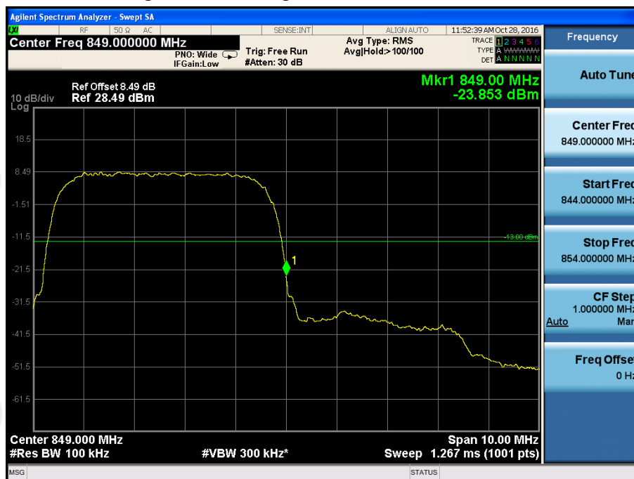
Higher Band Edge Plot on Channel 4233
