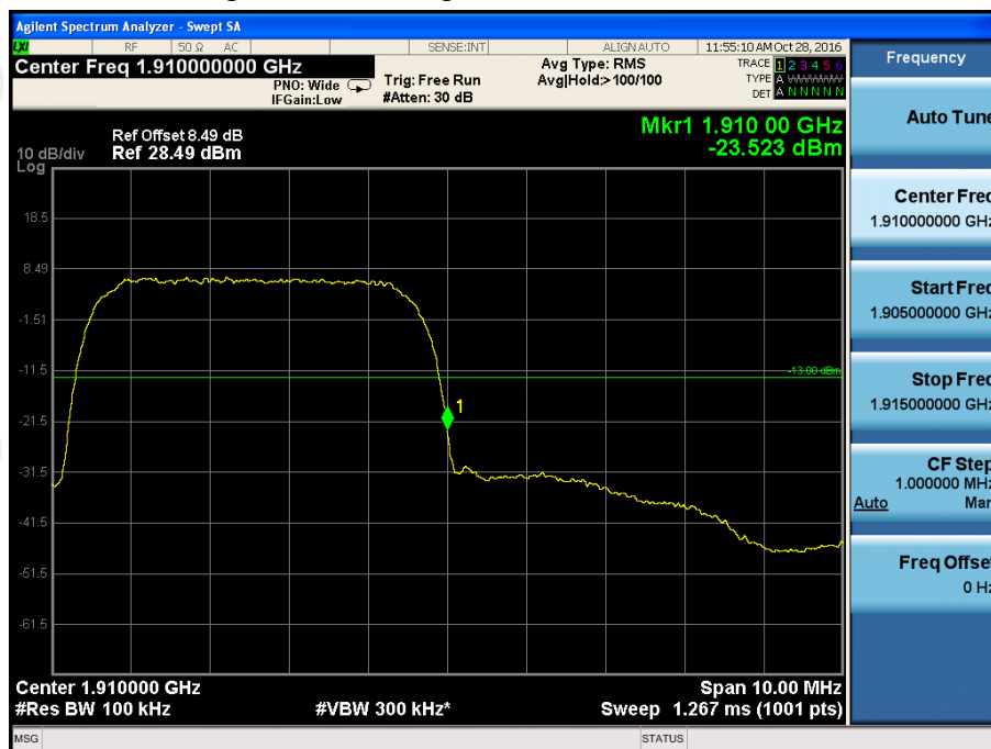
Higher Band Edge Plot on Channel 9538
