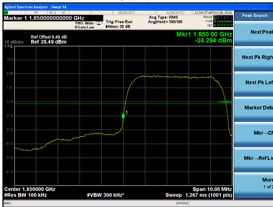
Higher Band Edge Plot on Channel 9538
