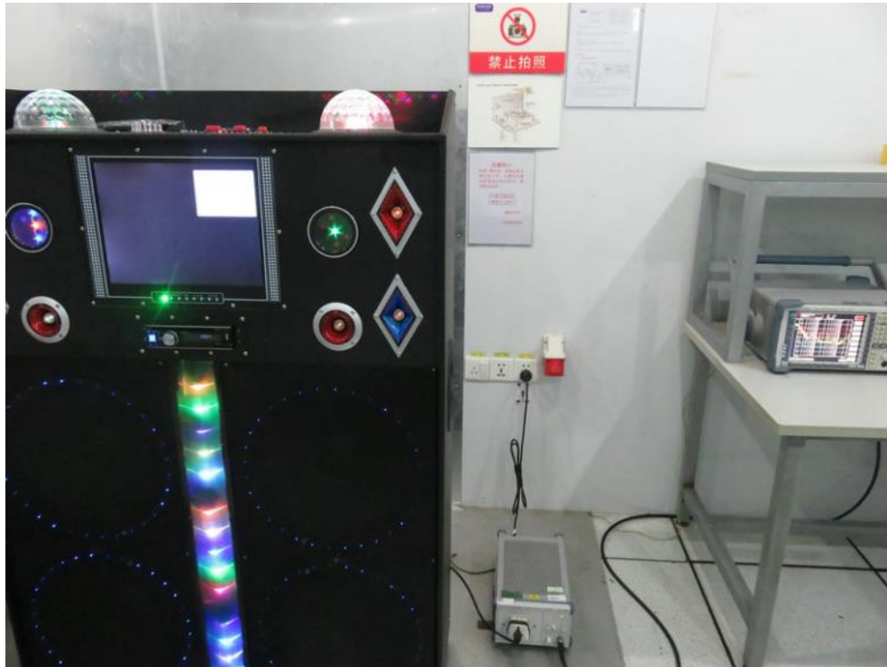
Photo of Conducted Emission Measurement
