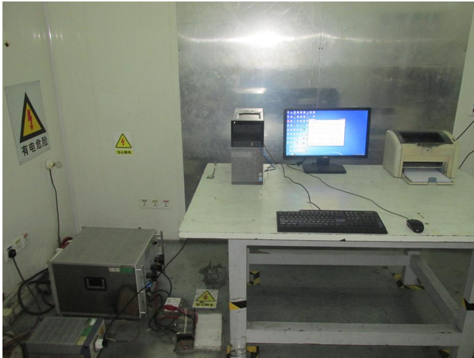
Photograph 6: Setup for Conducted emissions on AC Mains
