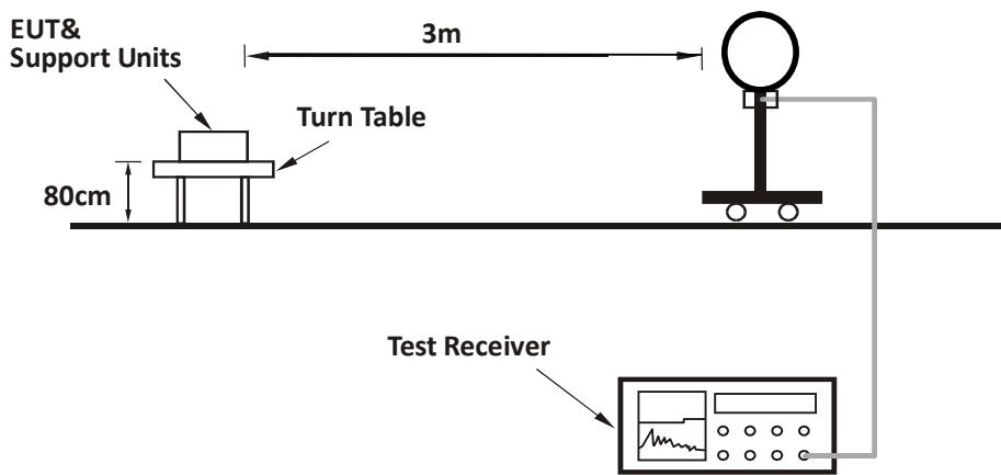
**For Radiated emission 30MHz to 1GHz:**
