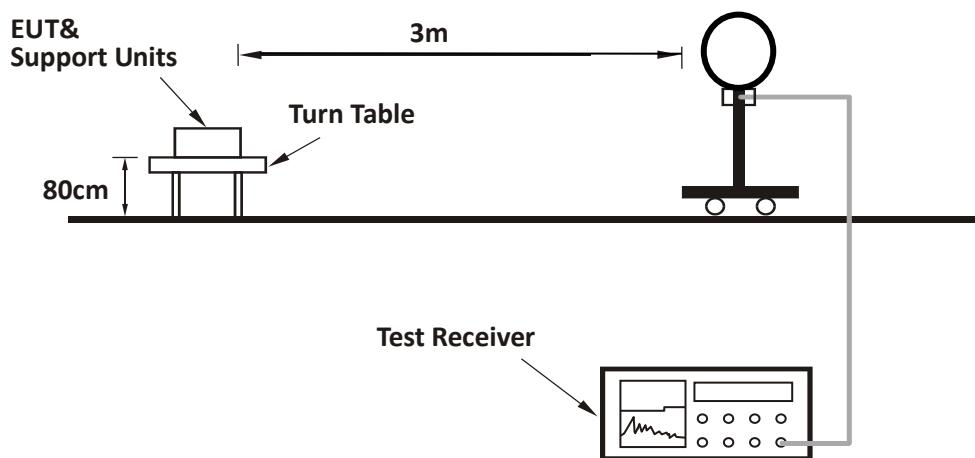
**For Radiated emission 30MHz to 1GHz:**
