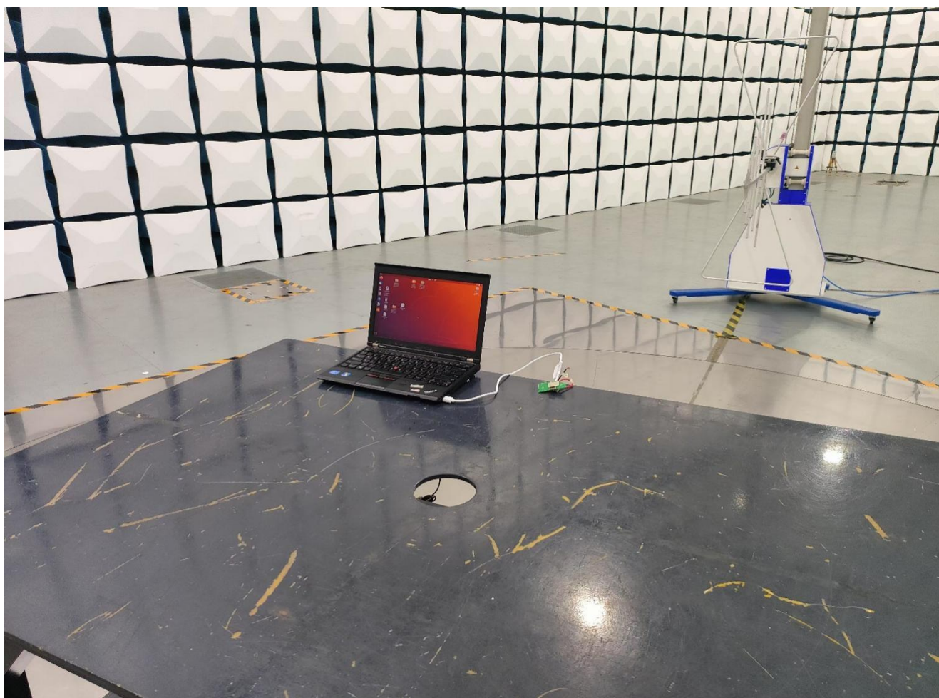
RF Radiated Test setup (30MHz~1GHz)
