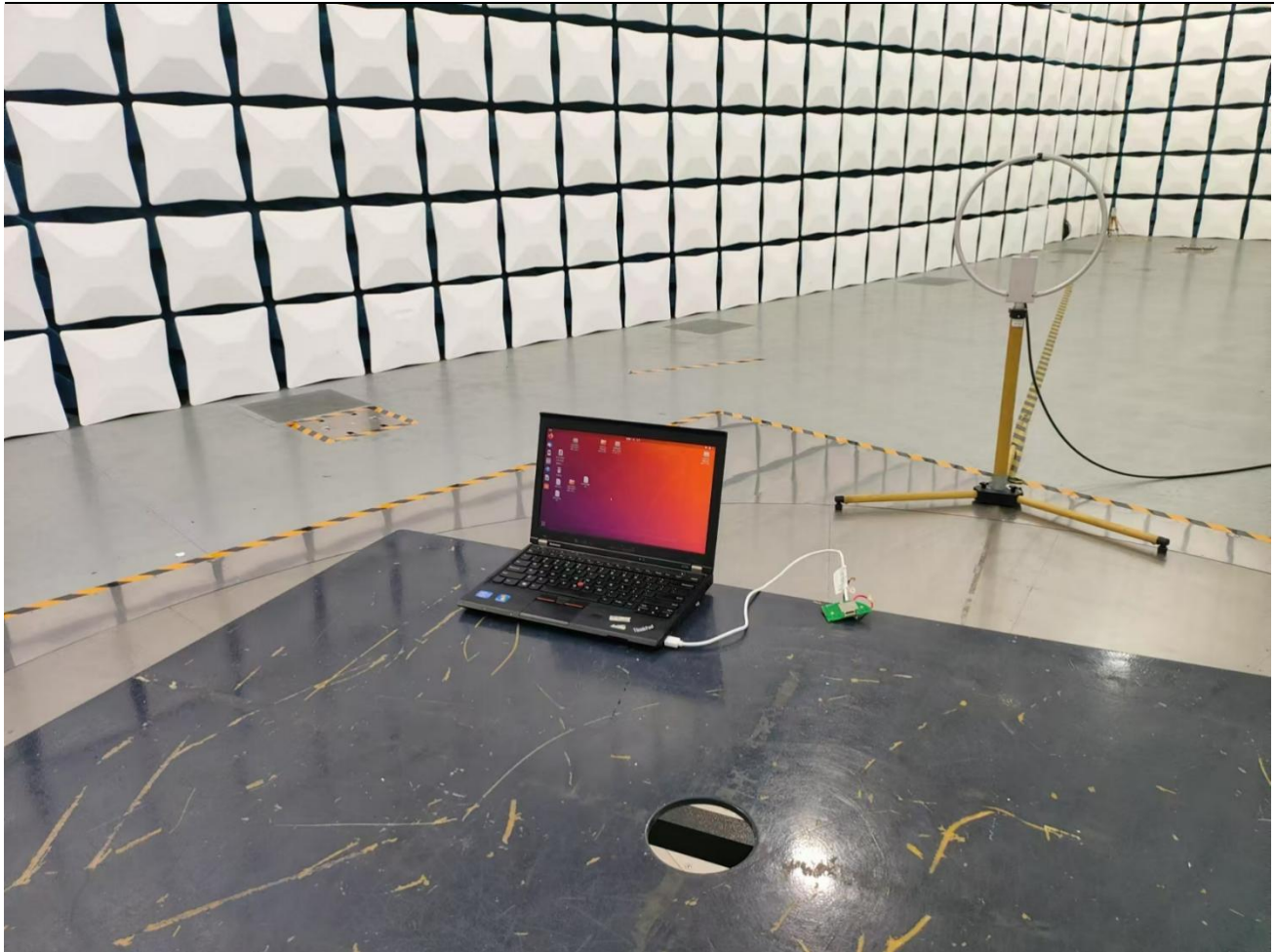
RF Radiated Test setup (9KHz~30MHz)
