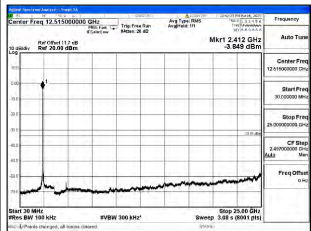
Mode:802.11n HT20 Frequency:2412MHz Ant:Chain1
