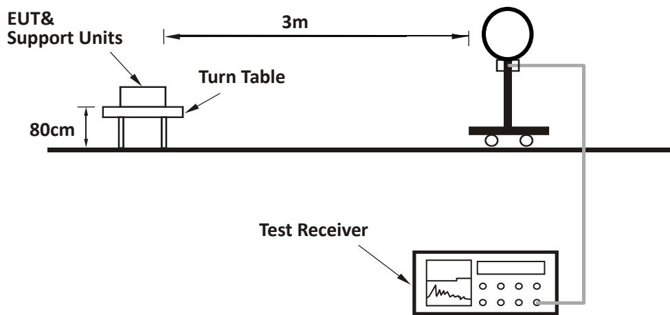
**For Radiated emission 30MHz to 1GHz:**
