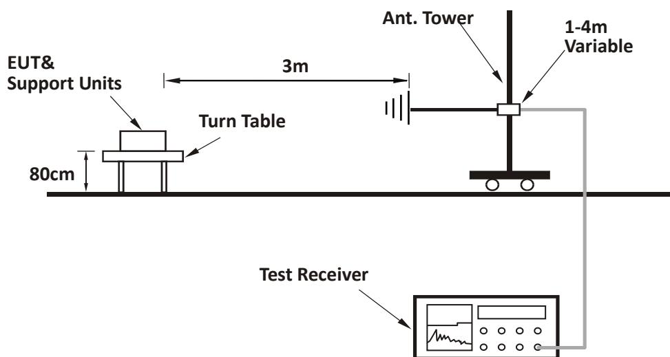
**TEST REPORT****For Radiated emission above 1GHz:**
