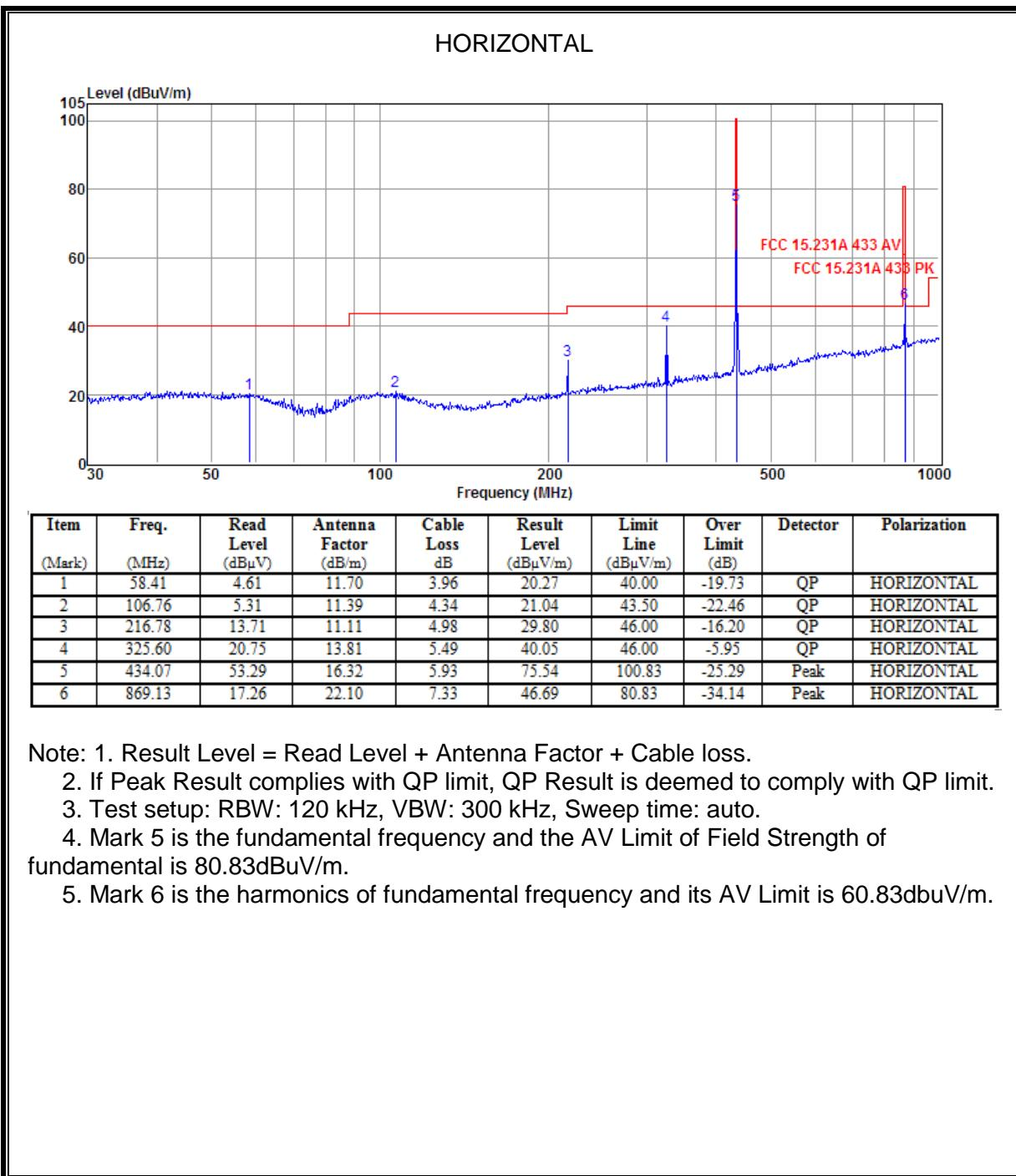
Note: 1. Result Level = Read Level + Antenna Factor + Cable loss.
