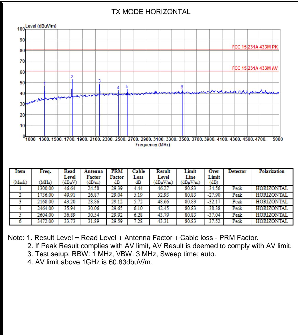
Note: 1. Result Level = Read Level + Antenna Factor + Cable loss - PRM Factor.
