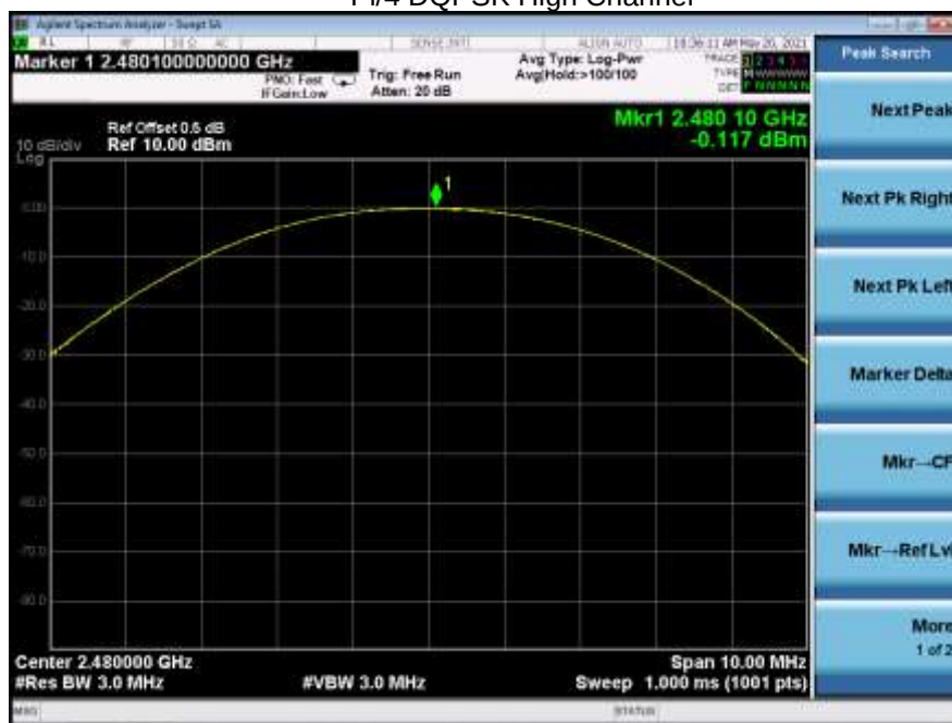
Pi/4 DQPSK High Channel
