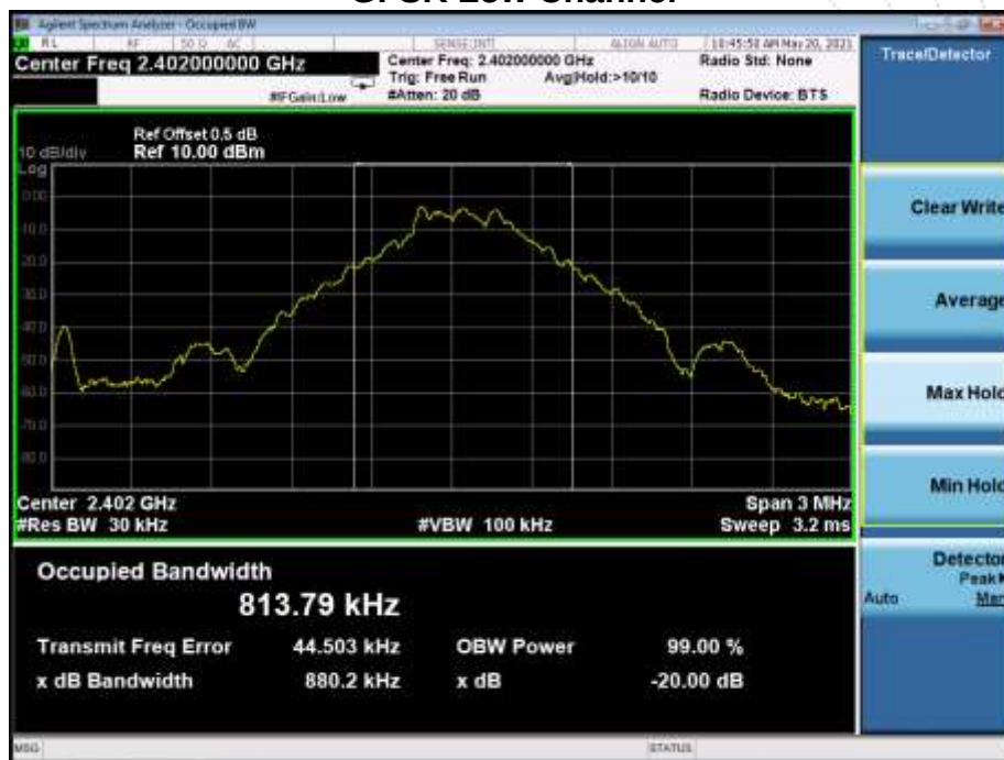
Test plots GFSK Low Channel
