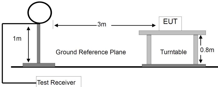
For Radiated Emission 30-1000MHz
