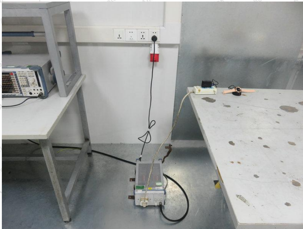
Photo of Power Line Conducted Emission Test
