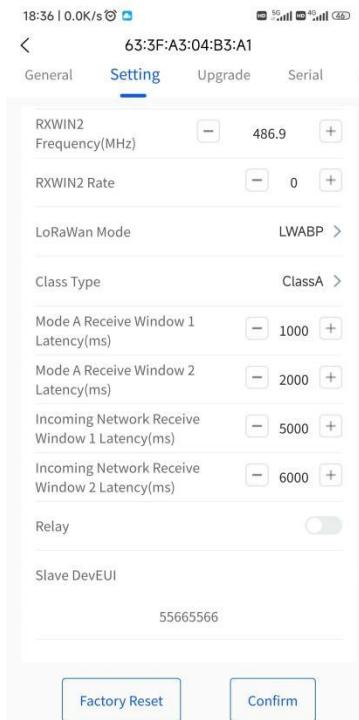
In the figure above, only one relay slave can be added at a time; in the figure, the slave with Devaddr 55665566 is added. You need to click Confirm for the changes to take effect. A maximum of 10 slaves can be added, and when more than 10, the addition failure will be prompted.
