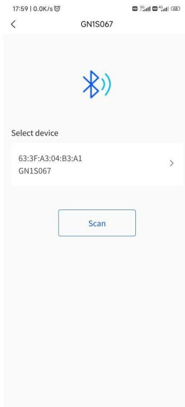
Click the scanned device to initiate a Bluetooth connection. If the connection is successful, you proceed to the next page, and the device's green light will flash to indicate a successful connection.
