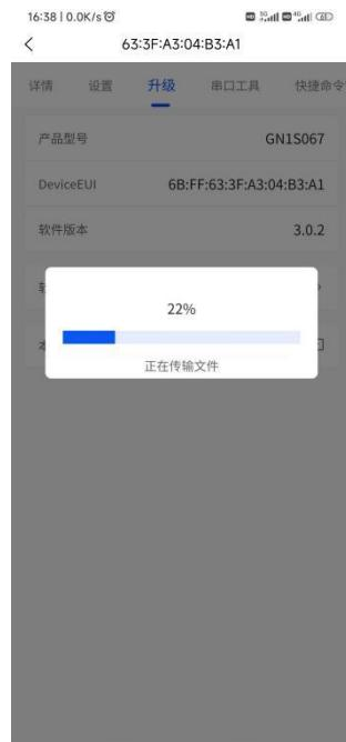
When the progress bar reaches 100%, the device will disconnect from the Bluetooth connection. After about 10 seconds, the device will complete the firmware update, and the blue light will stay on for 3 seconds. At this time, the APP can search the device again and initiate the connection.
