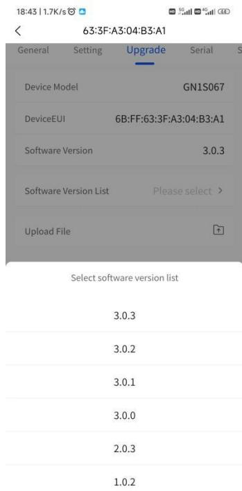
When you need to upgrade, select the corresponding software version number and confirm the upgrade. This process takes about 1 minute.
