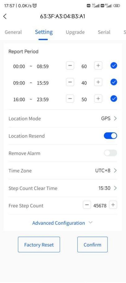
In this page, users can configure the report period, location resend function, time zone, step count clear time, and free step count (also known as GPS positioning exemption above). The location mode and the remove alarm need not be set and are reserved for future use.
