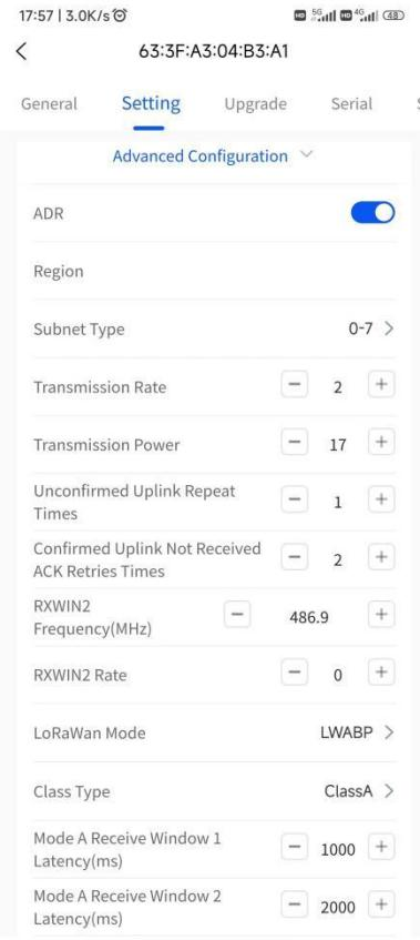
The parameters in the above figure are the parameters related to LoRaWAN network. Users who are not familiar with LoRaWAN should modify it carefully, as it may cause the device to lose contact.
