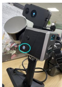
Press the start recording button, the scanner starts scanning
