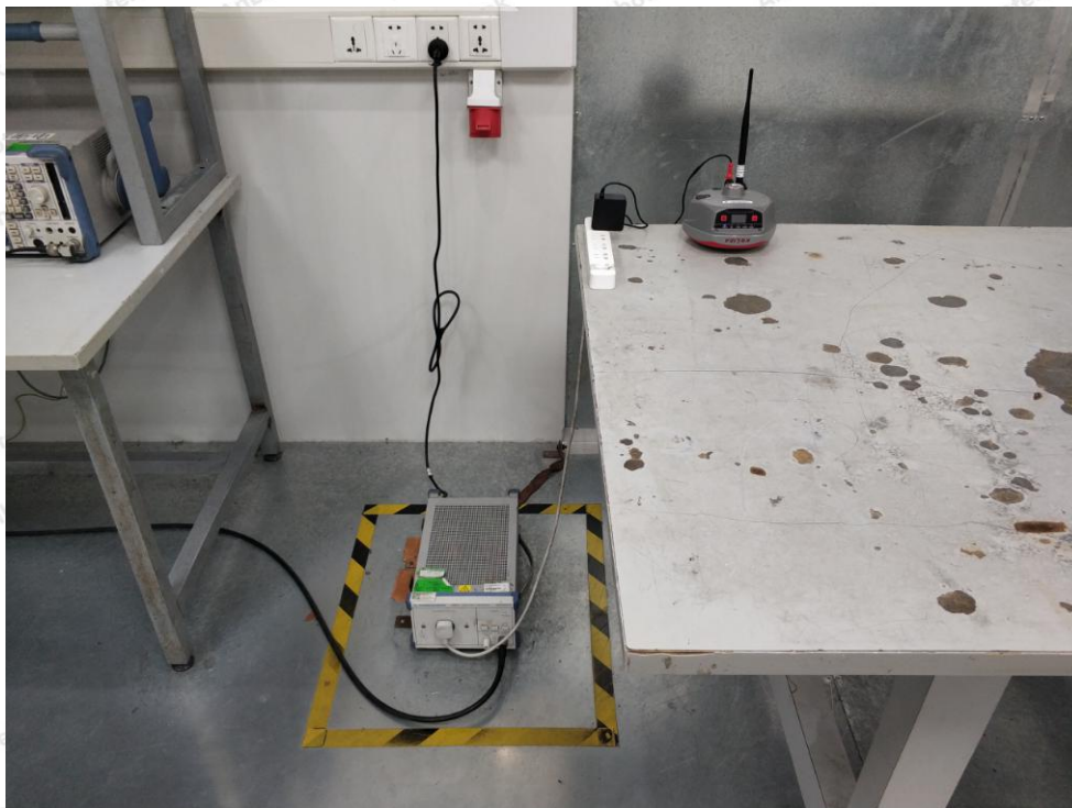
Photo of Conducted Emission Measurement
