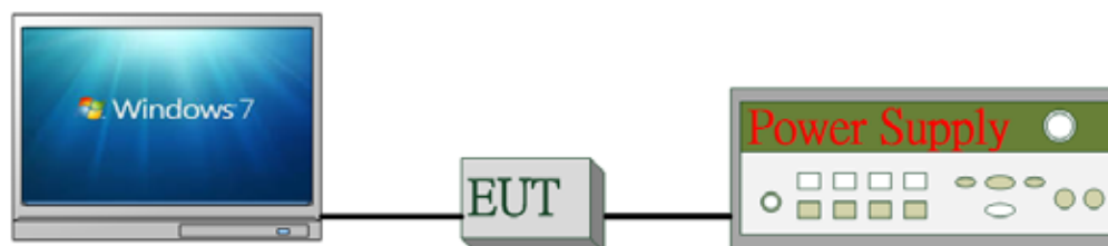
Fig. 2-2 Conducted (Antenna Port) Emission
