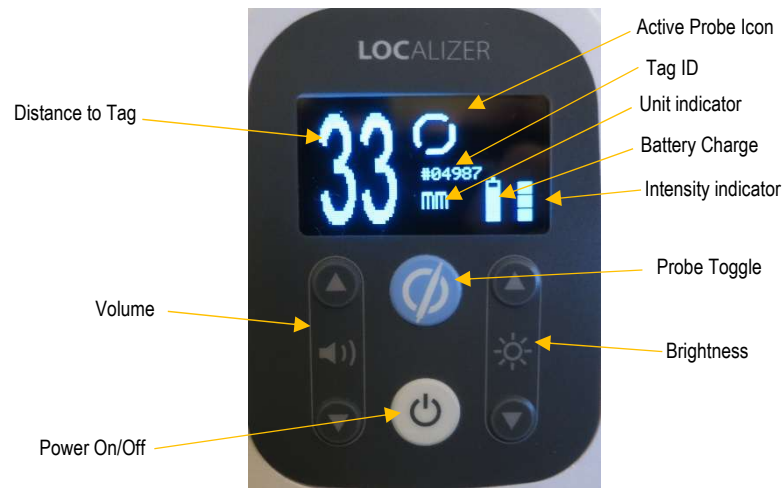
Figure 2. LOCALIZER Reader Controls and Displays (described below)
