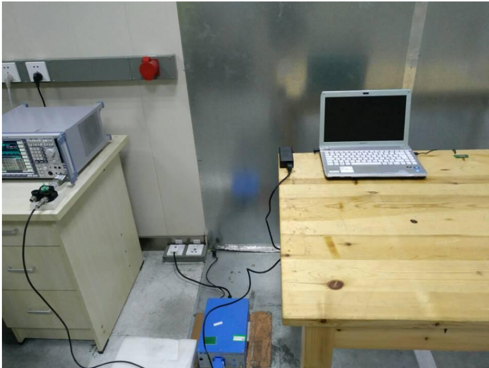
FCC RADIATED EMISSION TEST SETUP BELOW 1GHZ
