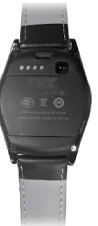
1. The back of the watch has four (4) magnetic pins that are used for charging the watch. To charge the watch each night, place with watch face down so the back of the watch is shown as illustrated in the photo on the left.
