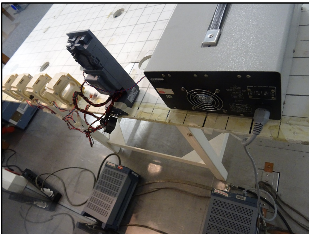
Photo 10: AC Conducted Emissions Test Setup
