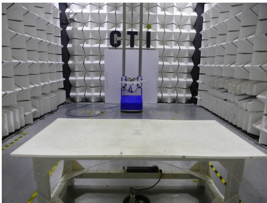
Radiated spurious emission Test Setup-2(30-1000MHz)
