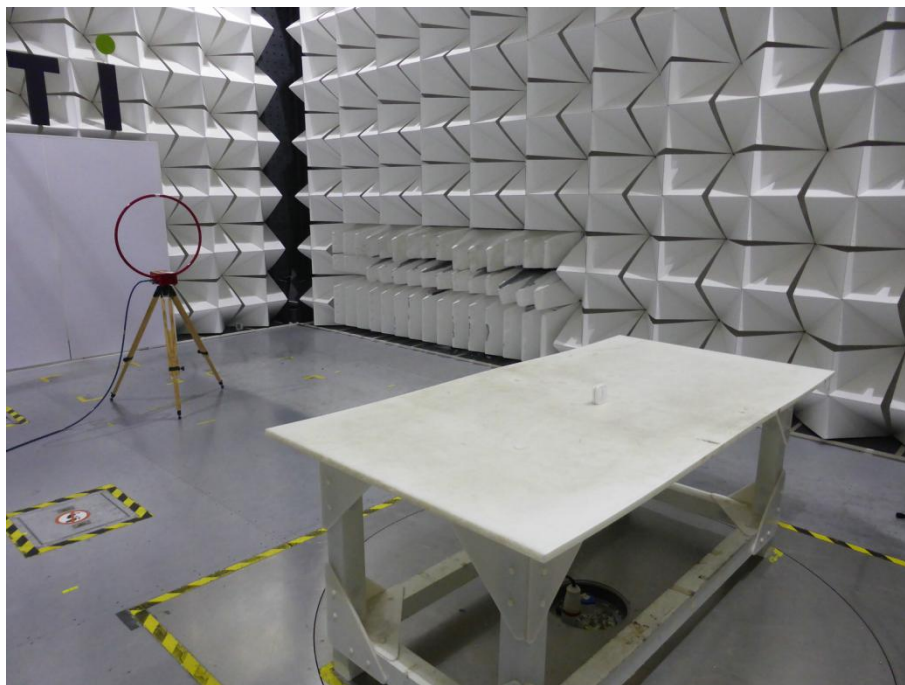
Radiated spurious emission Test Setup-1(Below 30MHz)
