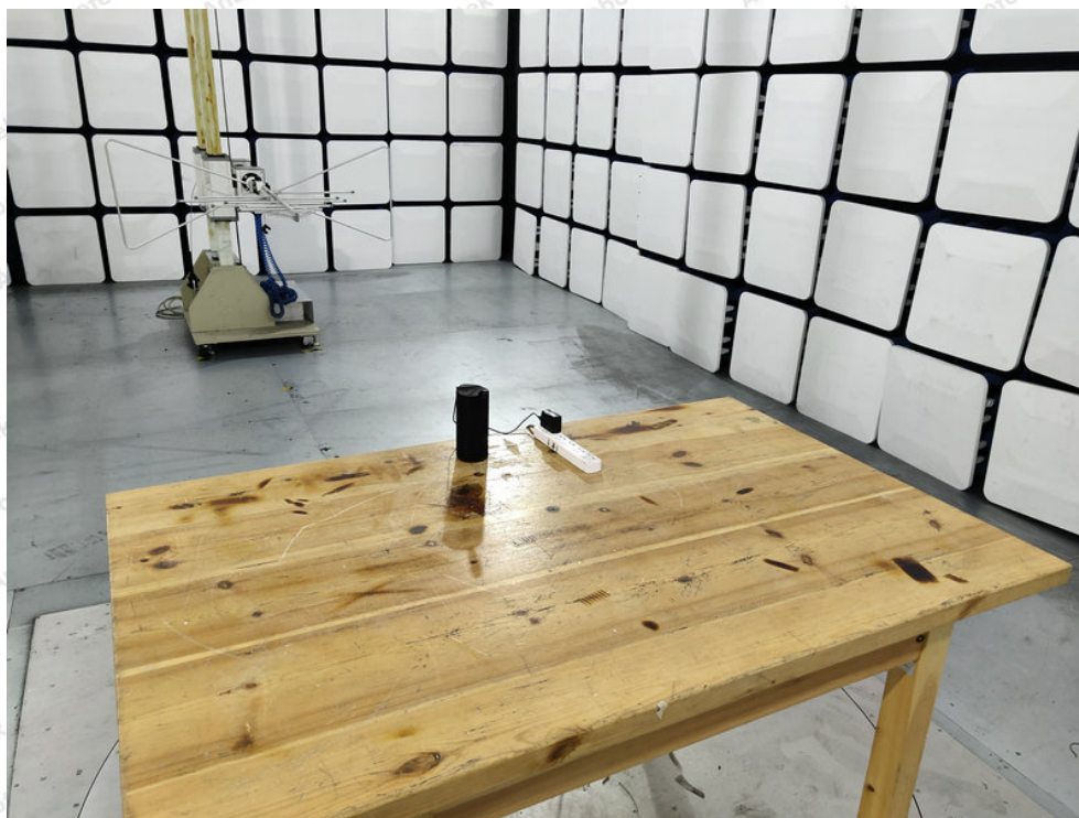
Photo of Radiation Emission Test
