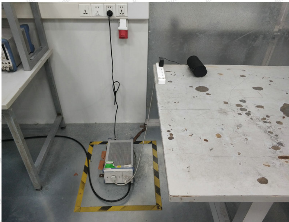
Photo of Conducted Emission Measurement
