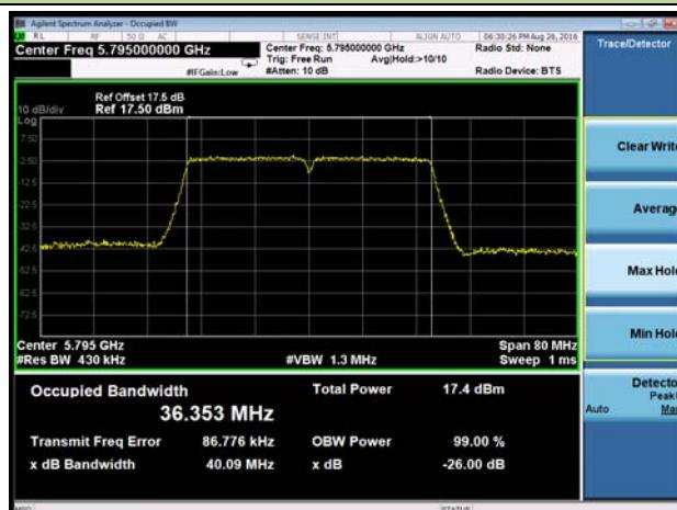
802.11ac-VHT20 26dB Bandwidth & 99% Bandwidth - Ant 0
