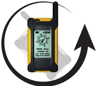
**Movement around the Z-Axis:** Hold the device in a horizontal position with the display facing up. Rotate the device in a circular motion (so the backside of the device is always facing the ground) until the counter has run out after 15 seconds. You may also place the device on a horizontal, flat and non metal surface for higher precision. A tone will indicate when the process is complete.
