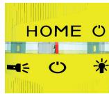
By bringing the upper ring in **„HOME“** position, the Marlin starts transmitting its position and a **HOME** signal. The **HOME** signal is intended to be a pickup call. It is received by every locating device (Ray and Basestation) that is within the same group as the Marlin that is transmitting. Devices of other groups won't show this signal.
