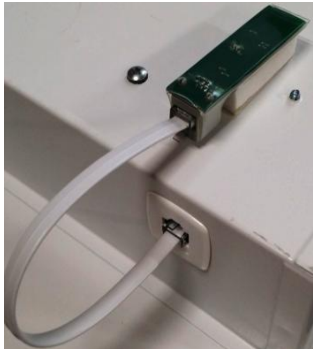
Figure 3: Backpack mounted to OR Controller P2 via luminaire panel mounted auxiliary port
