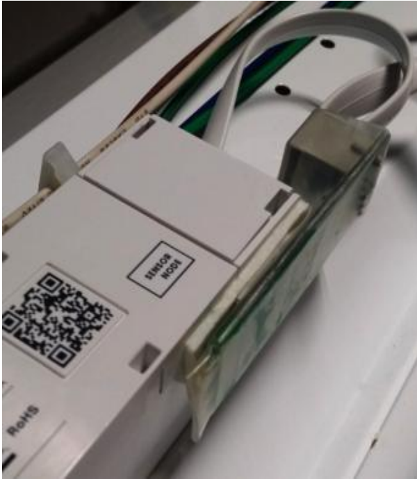
Figure 2: Backpack mounted direct to OR Controller P2
