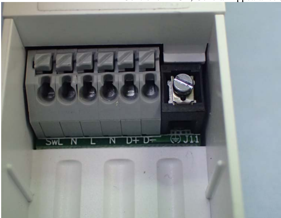
Figure 14 Controller P2UL, General Appearance (IO View)
