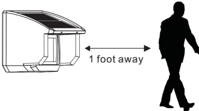
(the light of the ON/OFF button will flash once means the motion sensor was activated and sent the alarm signal; and then the motion sensor will back to work mode automatically after about 10 seconds if not detecting any movements)
