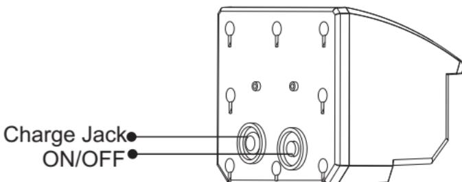
**Charge Jack:** used to connect the additional solar panel or DC 5V power adapter
