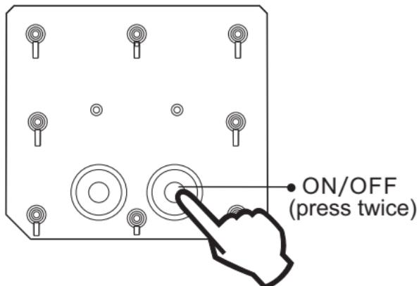
(the light of the ON/OFF button will flash once means the motion sensor was activated and sent the alarm signal)
