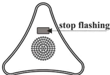
(a ring tone prompt and the indicator light stops flashing means the sensor has been added to the wireless alarm receiver successfully)
