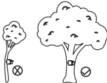
1. Please fix the motion sensor tightly to ensure the position and the direction will not be moved easily by wind.
