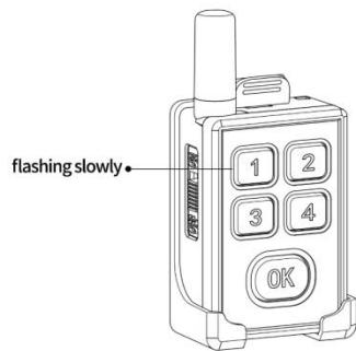
Ringtone/ vibrate /lights will be given out indicating that the sensor works with the portable reminder properly .(the alarm duration is based on the set of vibration duration, and if the vibration is turned off, the alarm duration is 1 minute)
