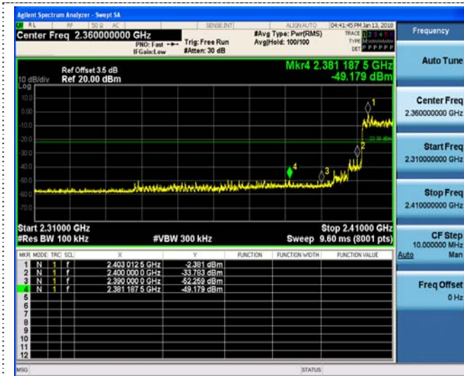
Left Band edge hopping on
