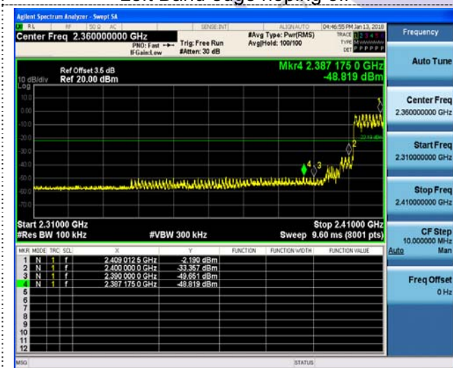
Left Band edge hopping on
