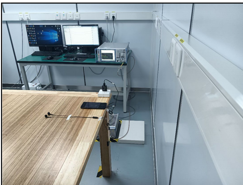
Fig. 4 Power line conducted emission setup photo
