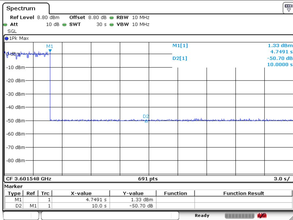
Bandwidth: 20MHz Setup with frequency 3680MHz and power level 20dBm/MHz
