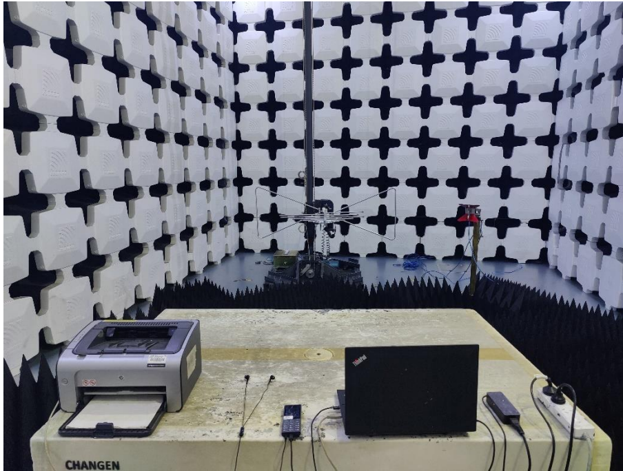
5. Radiated Emissions (Part 15B Data transfer, 1GHz-18GHz)
