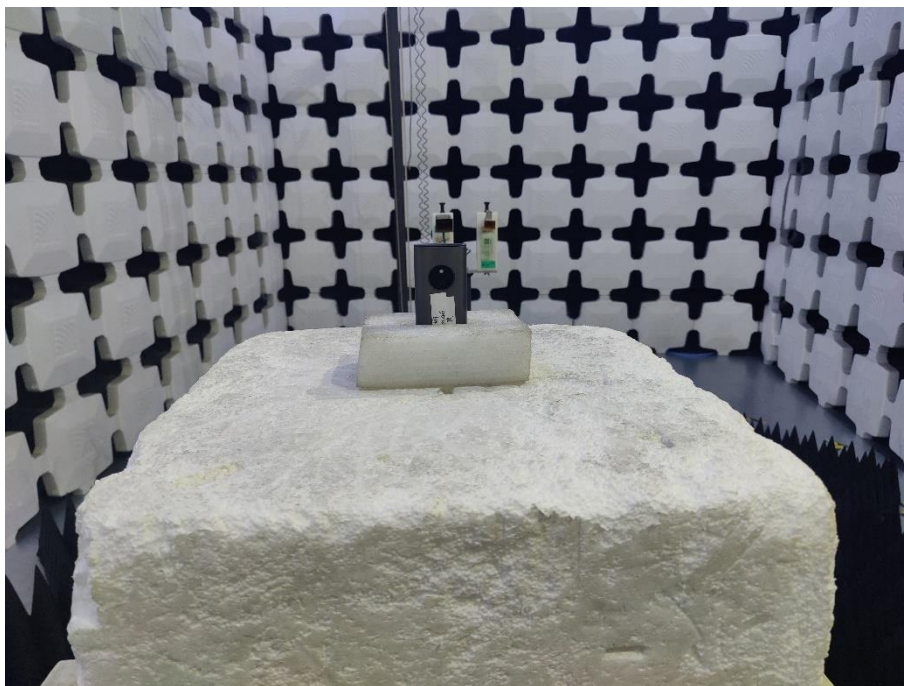
10. Radiated Emissions (Part 15C, 18GHz -26.5GHz)
