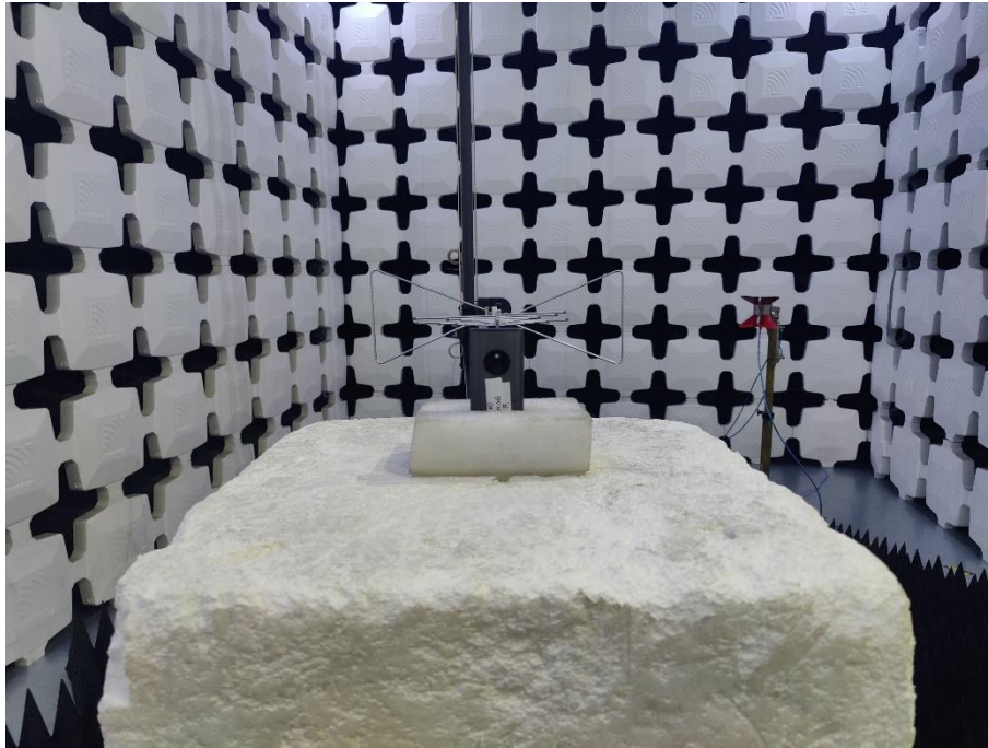
9. Radiated Emissions (Part 15C, 1GHz -18GHz)
