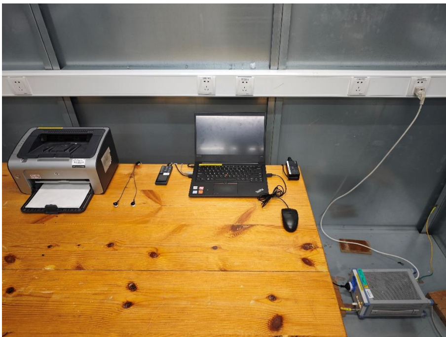
14. Conducted Emission (Part 15B, Data Transfer)
