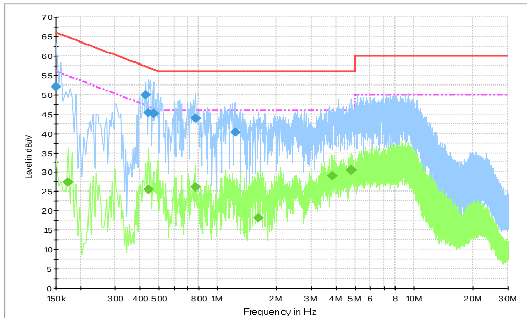
Fig. 23 AC Powerline Conducted Emission-Idle
