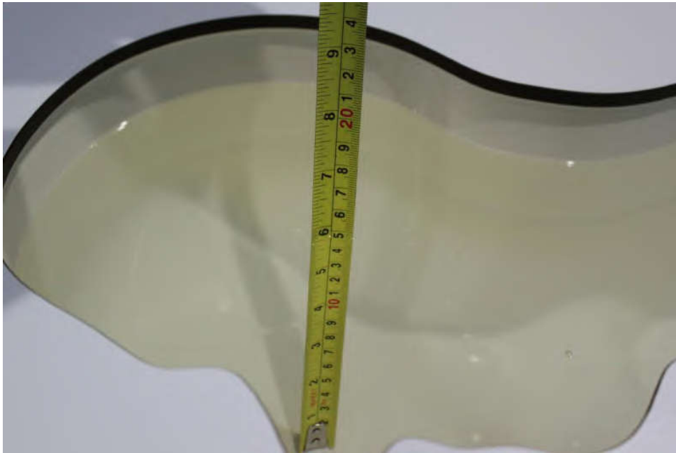
Picture 7-7: Liquid depth in the Head Phantom(5GHz)
